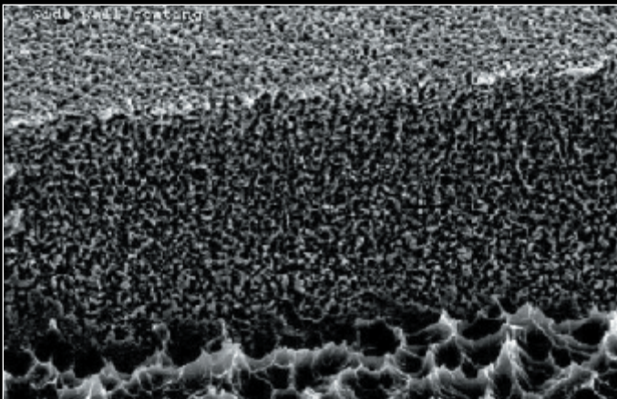
CO-BRA BOND ® HL Process microetches and coats both the circuit trace and sidewall of the trace, enhances resin flow and encapsulation, improves bond strength with higher performance resin systems.
