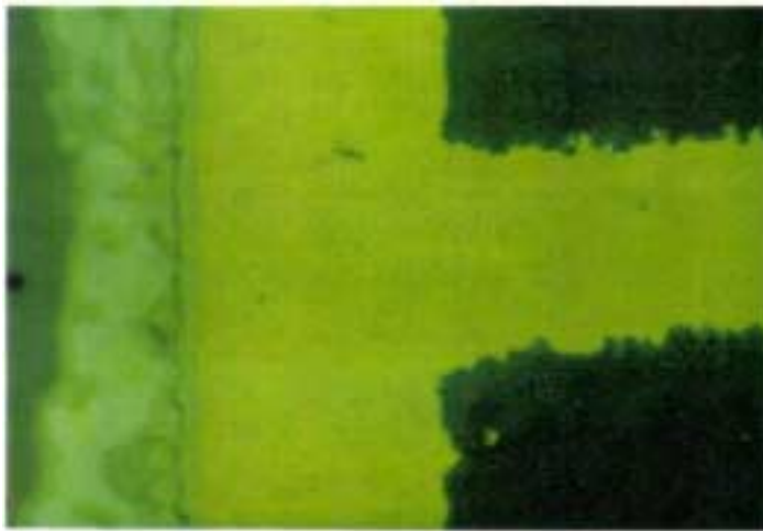
Figure 9 - PTH with Fixer – Copper to Copper Bond
